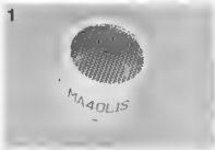
Photo 1. This is what a typical transducer looks like. Note that two different types are used in the transmitter end and the receiver.
