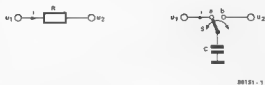
Figure 1. Resistor R in figure 1a may be replaced by the circuit in figure 1b, provided switch S switches to and fro between a and b at a sufficiently high frequency.
