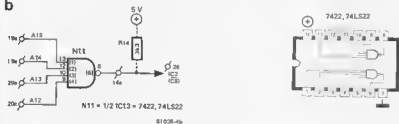
Figure 4. An alternative for figure 2 (two hardware possibilities) which provides further options with regard to the maximum amount of external memory. Only the EPROM address block including page FF is not to be used to avoid double addressing (see the article in the Elektor September issue).
