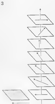
Figure 3. Portrayal of the molecular arrangement in a cholesteric liquid crystal. The arrow represents the direction of the molecule's long axis in each sheet.
