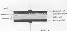
Figure 4. In the case of the electrolytic capacitor, the cathode plate is not only made up of metal foil, but also includes an electrolyte (electrically conductive fluid). The dielectric consists of aluminium oxide obtained through anodisation.
