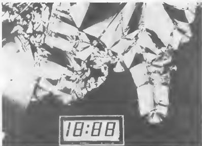
Photomicrograph of a smectic liquid crystal (see article on page 2) with a magnification of about 200. The liquid-crystal phase was formed by cooling a thin film of isotropic liquid (black background) and is highly ordered in spite of being able to flow. In other words, though liquid crystals are fluid they have some of the optical properties of solid crystals. This makes it possible, using nematic liquid crystals which can be electrically controlled, to produce the familiar sort of display seen in the lower part of the picture.
