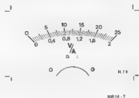
Figure 7. The new scale for the 1 mA moving coil meter.
