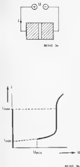
Figure 3. The structure of a Josephson junction (3a) and its voltage/current ratio curve (3b). The Josephson junction consists of two superconductors (shaded areas) with a very thin insulator, the Josephson barrier, between them.
