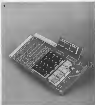
Photo 1. The completed Junior Computer looks like this. The keyboard and display can be clearly seen, the microprocessor and other components being on the other side of the printed circuit board.
