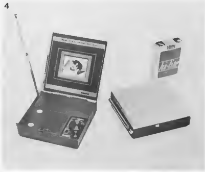
Photo 4. Liquid crystal screen in a pocket TV prototype manufactured by National Panasonic (Matsushita). With a total of 57,000 display dots it operates on a supply of 4.6 V.
