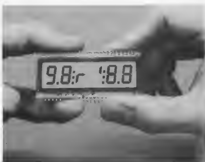
Figure 7. The current increase of LCD's is in linear proportion to the frequency. The segments represent a capacitive load.
