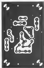
Figure 8. Printed circuit board and component lay-out for the amplifier of figure 7.
