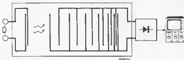
Figure 4. This type of SAW device, with ever-decreasing spacing of the 'fingers' in the output transducer, can be used for spectrum analysis of short signal 'bursts'.
