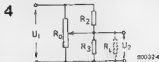
Figure 4. One or two fixed resistors can be added, between the wiper and one or both of the ends. The results can be surprising!
