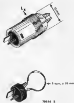
Figure 6. This figure shows how the coil is wound on the loudspeaker plug. The turns should be kept as far away as possible from the metal terminal pins of the plug in order to minimise energy losses.
