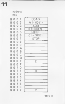
Figure 11. Showing how the programme to add x to y and store the result is held in the memory, together with the numbers x, y and the result z.
