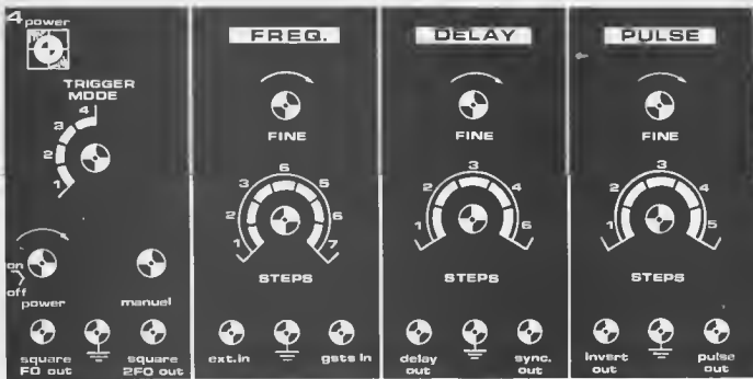
Figure 4. Suggested layout for the pulse generator front panel.
