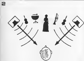
Figure 3. To properly reproduce the concert-hall experience four loudspeakers are needed, the front ones carrying the performer's sounds and the back ones cooperating with the front ones to reproduce the ambience.
